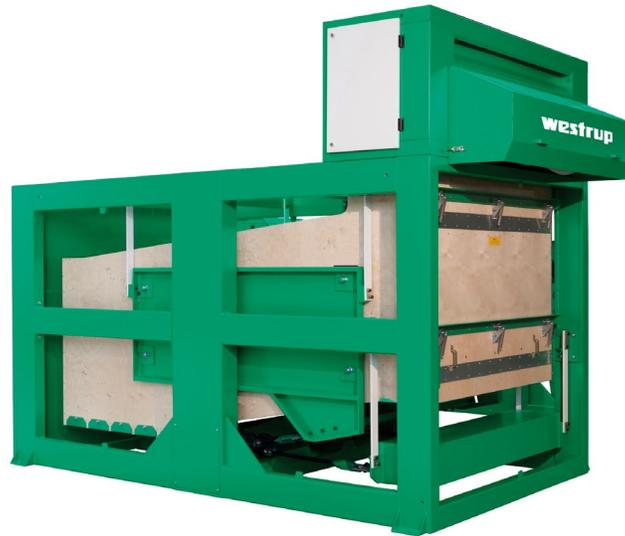
*The GD modular grader is a very compact machine ensuring an accurate sizing in 4 fractions of a large variety of products in one operation*
