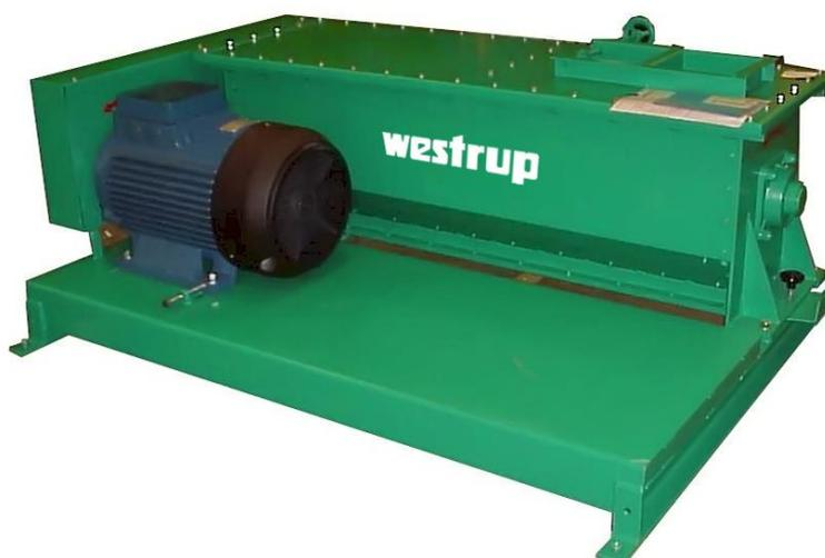
*The CW de-awner is used for pre-treatment of various grain types; the purpose of the de-awning operation is to remove awns from barley kernels, loose husks from wheat, and to clip oat kernels*
