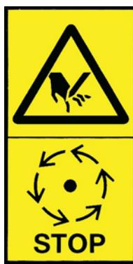
Rotating parts must only be touched when they are at a complete standstill.
