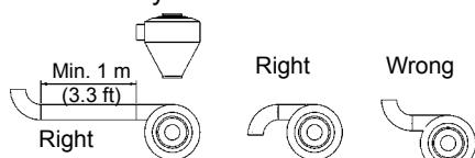
If it is necessary to install a bend prior to the cyclone, it shall bend in the same direction as the cyclone, or a straight pipe of minimum 1 m (3.3 ft) must be installed between them.
