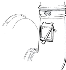
**Note: It is only necessary to lock the air intake regulator, if the reduction in amp consumption is demanded by the local power supply.**
