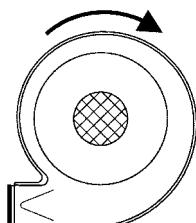
Please note, that the blowers TRL 20/40 (50Hz) and TRL 30/50 (60Hz) normally must not be operated without the use of a venturi. Otherwise, the motor can be overloaded. The venturi can, however, be left out if the air capacity of the blower is limited in a way that
