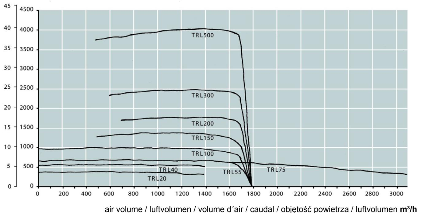
NB - the max. air volume delivered by the TRL blowers with air regulator is approximately 1.800  $m^3/h$  at different pressures depending on the type of blower. It is a general rule in pneumatic conveying that the higher pressure in the system, the higher the transfer rate.
