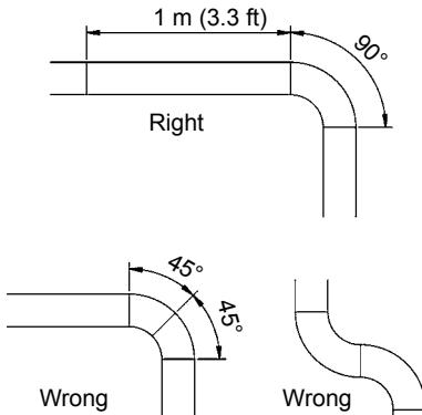
It is recommended to use a heavier 1 m (3.3 ft) pipe (OKR/OKD) following each bend to compensate for wear.
