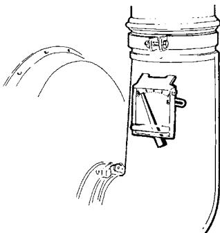
The intake regulator maintains a uniform air volume, even when the back pressure varies during operating. This ensures that the air velocity in a Kongskilde OK 160 pipe system constantly is approx. 25 m/sec. (56 mph), which is suitable for many pneumatic conveying purposes.
