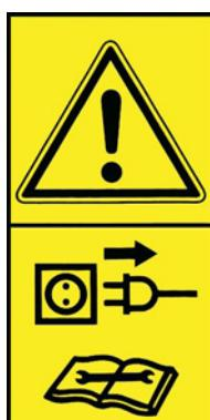
Always disconnect electricity prior to repairs and maintenance, and make sure that the blower cannot be started by mistake.
