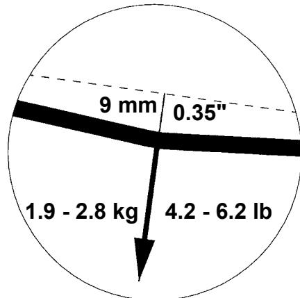
Check the tension of all the belts. In case it is not possible to adjust one set of belts, so that all the belts have the proper tension, the whole set must be replaced.
